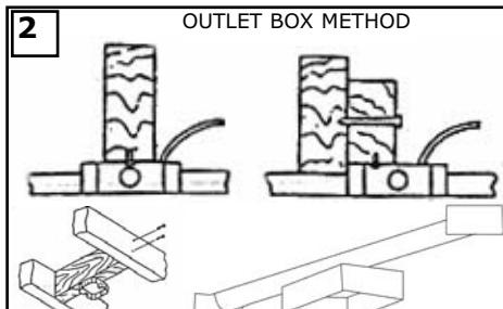
**Warning-Risk of fire, electric shock, or personal injury.** The fan in this box may be either directly supported from a structural framing member of a building and/or may be mounted to an outlet box marked acceptable for fan support of 31.8 kg (70 lbs) or less. Most outlet boxes commonly used for the support of luminaires may not be acceptable for fan support and may need to be replaced. Consult a qualified electrician if in doubt.
